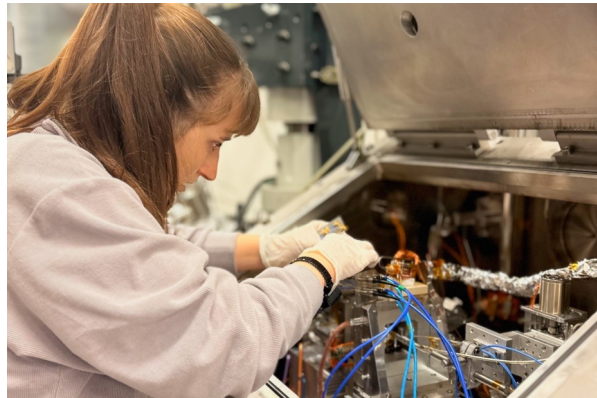
Fig. 2: Dr. Lisa-Marie Kern installing a sample at the MAXYMUS X-ray microscope.
