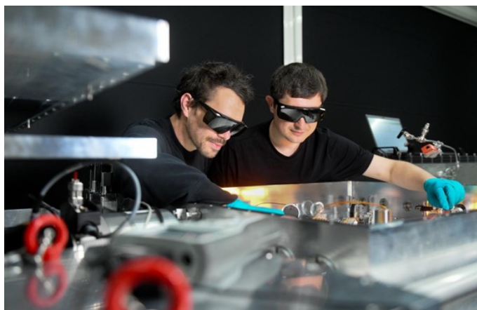
Fig. 1: Martin Kretschmar and Rostyslav Danylo with their setup for the generation of TW level, few-cycle laser pulses based on hollow-core fiber compression used for high-order harmonic generation.
