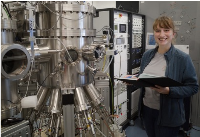
Fig. 1: Lisa Kern in front of the multi-source magnetron sputtering cluster used for the production of the GdFe film on \text{Si}_3\text{N}_4 membrane chips.
