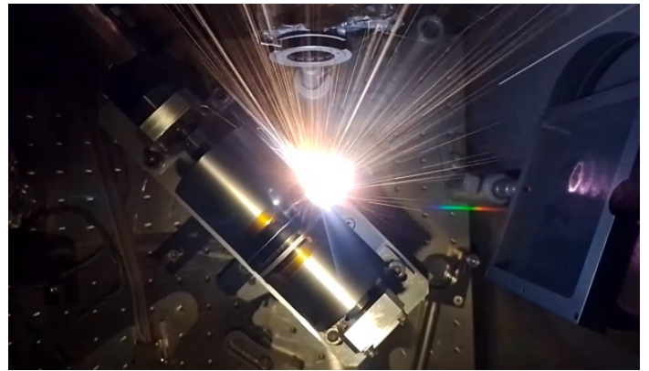
Fig. 2: Image of the plasma produced by an intense laser pulse on a rotating tungsten cylinder. From the plasma, soft X-rays are emitted [BBG23].
